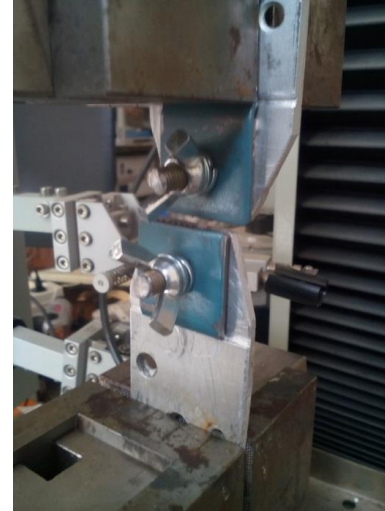
Zwick&Roell Z10 Maximum load force: 10 kN
