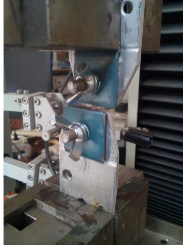
Specimen in the Zwick&Roell rupture machine
