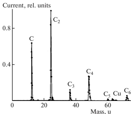
Fig. 4. Mass spectrum of negative ions produced in the sputtering ion source with the graphite sample.
