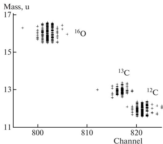
**Fig. 6.** Mass spectrum at the exit from the AMS under the conditions of scanning by the output magnet. On the abscissa axis, the time of flight of ions in the channels of the time-of-flight detector is plotted.
