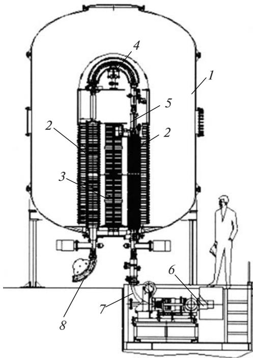
**Fig. 1.** Accelerator mass spectrometer: (1) tank for SF<sub>6</sub>, (2) accelerating tube, (3) electrostatic filter, (5) magnesium vapor target, (6) ion source, and (7, 8) magnetic filters.
