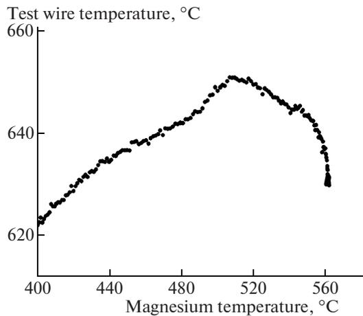
Fig. 3. Test of the magnesium vapor target. The temperature of the wire strained in the stripping channel is plotted vs. the temperature of the magnesium container.
