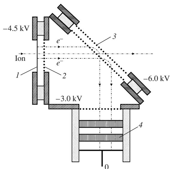
**Fig. 1.** Time-of-flight detector: (1) film, (2) accelerating grid, (3) electrostatic mirror, and (4) MCP.
