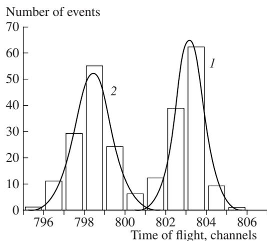
**Fig. 3.** Ion TOF distribution (0.5 ns per channel) (1) without a film and (2) with an additional film at the detector input.
