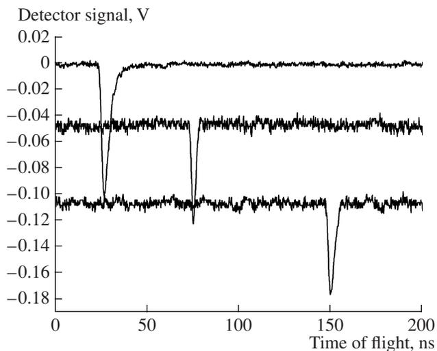
**Fig. 2.** Signals of three TOF detectors sequentially passed by an ion with an energy of 1 MeV.
