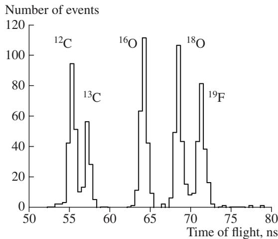
Fig. 5. Spectrum of time intervals for a mixed ion beam.
