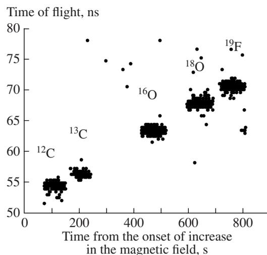
**Fig. 4.** Sequential changes in the time of flight with a change in the magnetic field in the spectrometer's output magnet.
