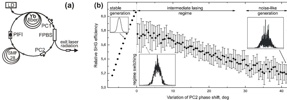
**Fig. 1** (a) Laser layout (PC – polarization controller, PIFI – polarization-independent fiber isolator, FPBS – fiber polarization beam splitter, LD – pump laser diode) and (b) simulated relative second harmonic generation efficiency for different generation regimes as a function of PC2 phase shift. Insets show temporal intensity distributions for stable, intermediate and noise-like generation regimes.
