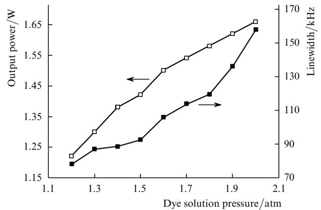
**Figure 3.** Dependences of the linewidth and output power of the dye laser on the dye solution pressure at the nozzle entrance.
