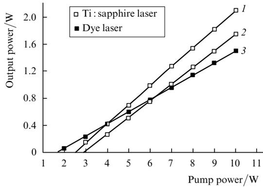
**Figure 7.** Dependences of the maximum output power of the combined laser on the pump power: (1) Ti:sapphire laser with the crystal and optics of the best quality; (2, 3) typical lasers.
