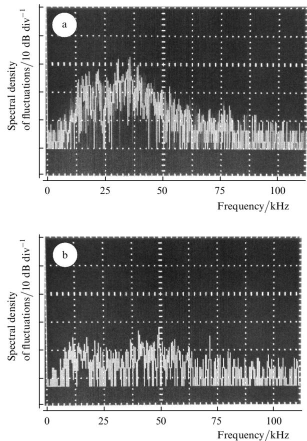
**Figure 4.** Density spectra of residual fluctuations of the emission frequency of the dye laser with a quartz nozzle with the output slit of size 3.5 mm  $\times$  0.25 mm (a) and a sapphire nozzle with the slit of size 5 mm  $\times$  0.3 mm (b).
