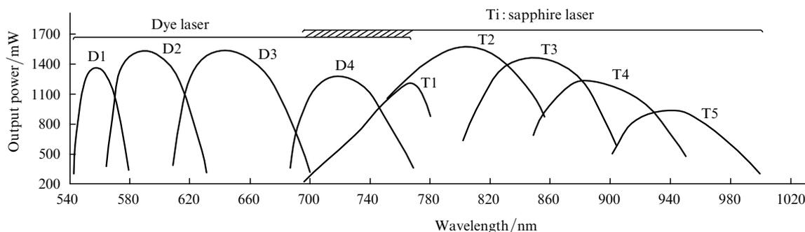
**Figure 6.** Tuning curves of the single-frequency combined laser for different dyes [rhodamine 110 (D1), rhodamine 6G (D2), DCM (D3), and pyridine 2 (D4)] and five mirror sets [T1 (695–780 nm), T2 (750–850 nm), T3 (800–900 nm), T4 (850–950 nm), and T5 (900–1000 nm)].
