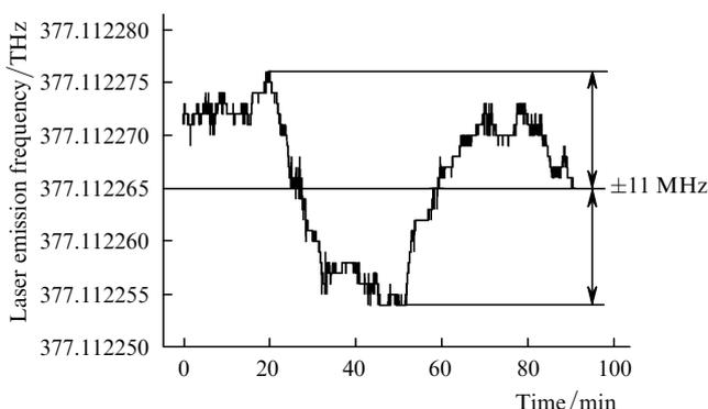
**Figure 5.** Time dependence of the laser emission frequency recorded with a WS/Ulimate wavemeter.
