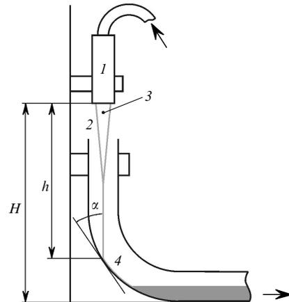
**Figure 2.** Geometry of the vertical dye solution jet in the laser: (1) nozzle; (2) dye jet; (3) point of incidence of the pump beam on the jet; (4) drain tube; ( $h$ ) distance from the nozzle to the point of incidence of the dye jet on the drain tube; ( $H$ ) height of the nozzle above the reference plane.
