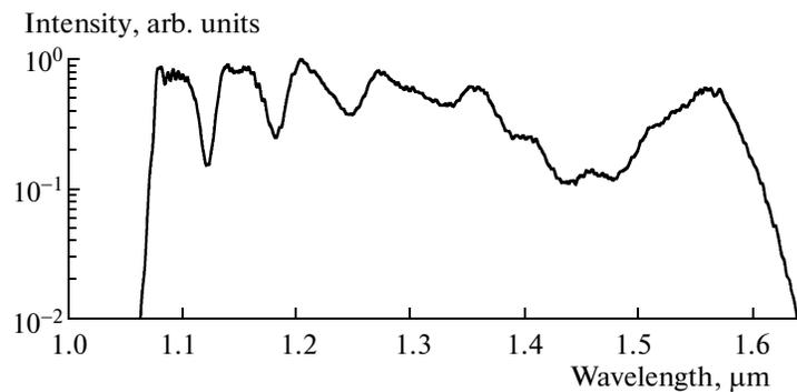
**Fig. 3.** The spectrum of the Raman-dominated supercontinuum at the exit of the 1060-XP fiber.
