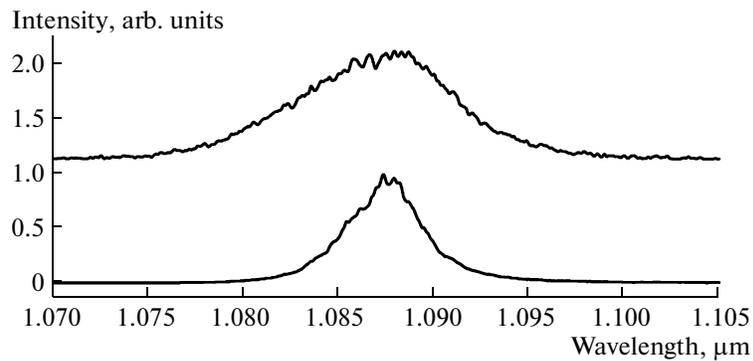
**Fig. 2.** Spectra of (lower curve) the laser radiation and (upper curve) the amplified radiation.
