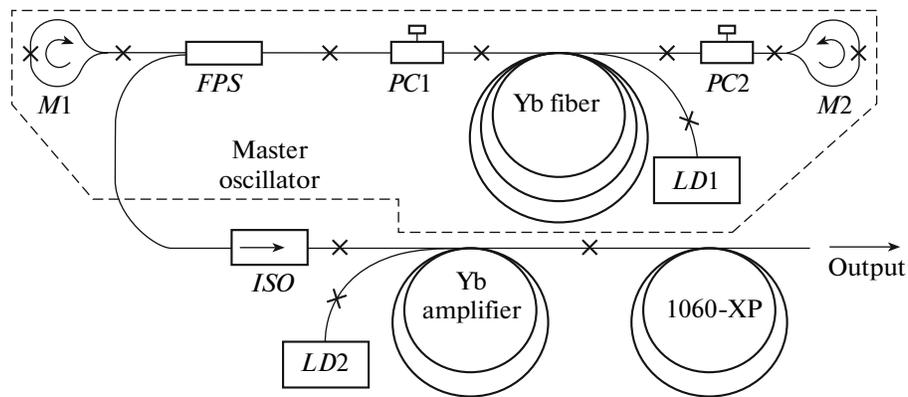
**Fig. 1.** Scheme of the all-fiber supercontinuum generator: *LD1* and *LD2* pumping laser diodes with a wavelength of 975 nm, *PC1* and *PC2* polarization controllers, *M1* and *M2* broadband fiber reflectors, *FPS* fiber polarization splitter, and *ISO* optical isolator.
