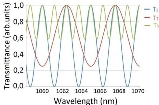
Fig.2 Calculation of fiber birefringent filter with different parameters
