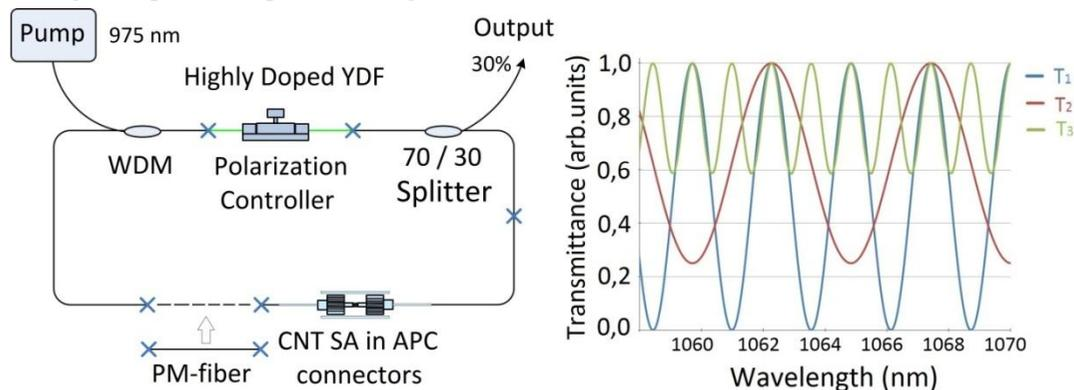
Fig.1 The scheme of Yb mode-locked laser with a SWCNT-based SA.
