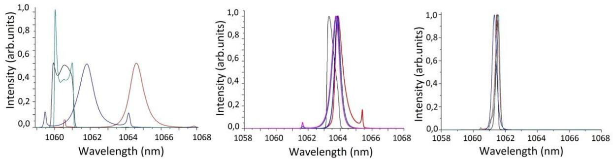
Fig.3 Emission spectra of Yb mode-locked fiber laser for different lengths of PM-fibers and different settings of polarization controller.
